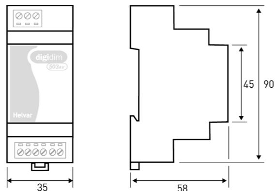
DIN rail housing; Width of 2 modules. Weight 80 g
