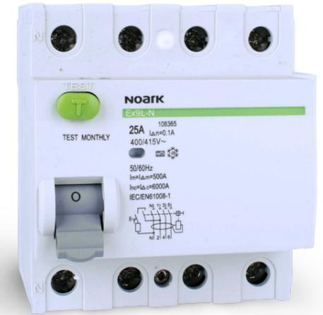
Ex9L-N residual current circuit breakers are suitable mainly for domestic applications. They are based on permanent magnet principle. It brings the advantage of Voltage independent function. Adequate voltage is only necessary when testing the RCCB with the T test button. Magnetic RCCBs should be tested regularly with a period of one month. 6 kA variant of the Ex9L-N residual current circuit breaker is intended mainly for low demanding application like basic protection in household installations.
