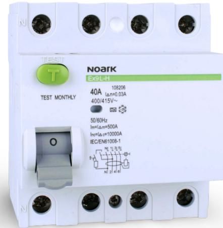
Ex9L-H residual current circuit breakers are suitable for domestic as well as industrial applications. They are based on permanent magnet principle. It brings the advantage of voltage independent function. Adequate voltage is only necessary when testing the RCCB with the test button. Magnetic RCCBs should be tested regularly with a period of one month.
