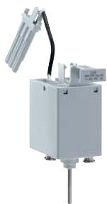
Undervoltage releases are devices which are generally controlled by an N/C type contact. The trigger instantaneous opening of the circuit breaker if their supply voltage drops below a certain threshold and in particular if the control contact opens. These releases are equipped with a device for limiting their consumption after the circuit has been closed.
