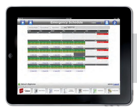
Using the scheduler Emergency testing can be fully automated with reports being generated in PDF format which can be emailed.
