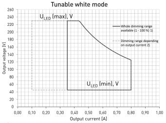
1) From 350 mA to 800 mA, full dimming range (  $1\,\%$  –  $100\,\%$  ) and wide CCT dynamic range available in the whole area. Each single channel can dim down to 0.50 mA level.
