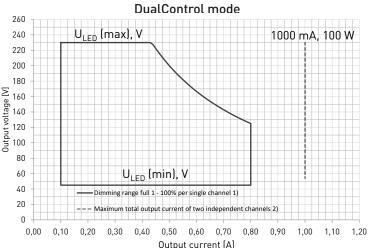
1) Full 1 - 100 % dimming range provided on whole operation window. Each single channel can go down to 1 % dimming at 100 - 800 mA.
