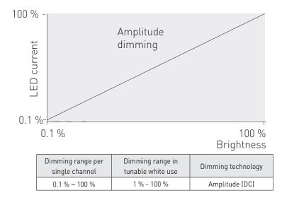
LL100iC-DA-100-800 LED driver implements amplitude dimming technology across whole dimming range. Amplitude dimming offers the best available technology for dimming the light output in an accurate and flicker-free way to ensure high quality lighting in even the most demanding situations such as camera recording applications. Amplitude dimming technology complies with IEEE 1789-2015 recommendations of current modulation to mitigate health risks to viewers.
