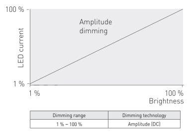
LL120HE-DA-200-900-IND LED driver implements amplitude dimming technology across whole dimming range. Amplitude dimming offers the best available technology for dimming the light output in an accurate and flicker-free way to ensure high quality lighting in even the most demanding situations such as camera recording applications. Amplitude dimming technology complies with IEEE 1789-2015 recommendations of current modulation to mitigate health risks to viewers.
