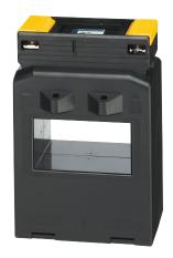
SOCOMEC current transformers deliver a standard secondary current that is proportional to the primary current and suitable for the rating of the associated energy meter. They are equipped as standard with removable terminal covers and double terminals allowing the secondary to be short-circuited without any risk.
