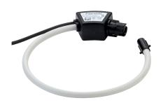
TF flexible current sensors measure the load currents of an electrical circuit and send the data to meters and Power Monitoring Devices or current modules via an RJ12 plug-and-play connection. Thanks to a wide measurement range, TF current sensors cover a wide current range from 100 to 6000 A, with only 7 references. TF flexible current sensors can be used with DIRIS Digiware I modules, DIRIS A-40 and DIRIS B.
