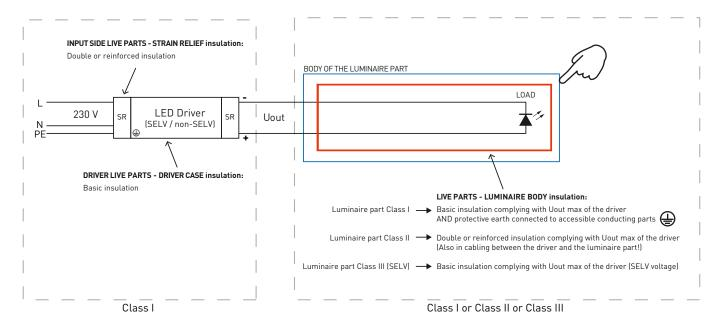
Note: The combination is Class I, even though Class II or Class III luminaire parts are used!
