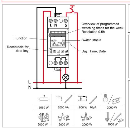
Operating principle: Type 1.B. S. T. IEC/EN 60730-1, IEC/EN 60730-2-7 Operation in a normal environment
