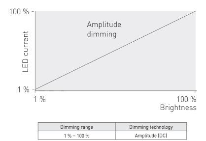
LC44MINI-DA-700-1050 LED driver implements amplitude dimming technology across whole dimming range. Amplitude dimming offers the best available technology for dimming the light output in an accurate and flicker-free way to ensure high quality lighting in even the most demanding situations such as camera recording applications. Amplitude dimming technology complies with IEEE 1789-2015 recommendations of current modulation to mitigate health risks to viewers.
