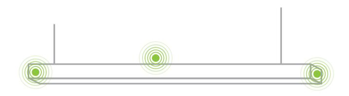
**IN OR OUT?** The Node is designed to be mounted freely anywhere inside or outside the luminaire. This is the best way to ensure connectivity in different luminaire designs or installation sites.
