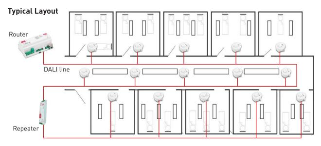
Note: This solution does not provide additional DALI addresses. The DALI limit of 64 addresses still applies.
