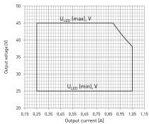
Note: Dimming between 1-100 % is possible across the operating window, restricted by the absolute minimum current of 5 mA.
