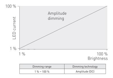
LC51SE-DA-900-1400-LOOP driver implements amplitude dimming technology across whole dimming range. Amplitude dimming offers the best available technology for dimming the light output in an accurate and flicker-free way to ensure high quality lighting in even the most demanding situations such as camera recording applications. Amplitude dimming technology complies with IEEE 1789-2015 recommendations of current modulation to mitigate health risks to viewers.
