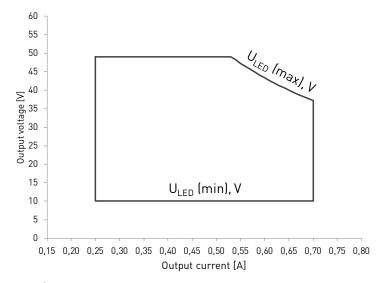
Note: 1) Dimming between 1 % - 100 % possible across the operating window, restricted by the absolute minimum dimming current of 7 mA.
