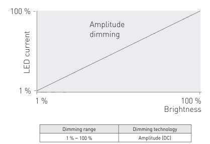
LC26MINI-DA-250-700-SR LED driver implements amplitude dimming technology across whole dimming range. Amplitude dimming offers the best available technology for dimming the light output in an accurate and flicker-free way to ensure high quality lighting in even the most demanding situations such as camera recording applications. Amplitude dimming technology complies with IEEE 1789-2015 recommendations of current modulation to mitigate health risks to viewers.
