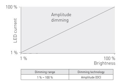
LL50SE-DA-100-1400 LED driver implements amplitude dimming technology across whole dimming range. Amplitude dimming offers the best available technology for dimming the light output in an accurate and flicker-free way to ensure high quality lighting in even the most demanding situations such as camera recording applications. Amplitude dimming technology complies with IEEE 1789-2015 recommendations of current modulation to mitigate health risks to viewers.
