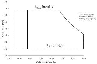
1) From 350 mA to 1400 mA, full dimming range (  $1\,\%$  -  $100\,\%$  ) available in the whole area. 2) From 100 mA to 350 mA, the absolute minimum dimming level is limited to 3.5 mA.
