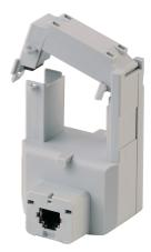
The split-core current sensors in the TR ranges enable the current of an electrical installation to be measured. Used with power monitorign device DIRIS Digiware, DIRIS A-40, DIRIS B, they make it possible to perform measurements between 25 and 600 A, with guaranteed accuracy. The RJ12 connection provides quick connections, and the integrated intelligence prevents any configuration errors.
