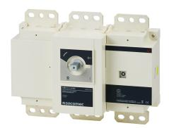
SIRCO AC units are manual or motorised multi-pole load break switches. They make and break under load conditions and provide safety isolation. SIRCO AC devices are designed for extreme applications up to 690 VAC -AC 23.
