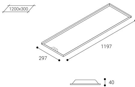
Installation: Keep a minimum 50 mm security distance between the luminaire and the ceiling to ensure its correct performance.
