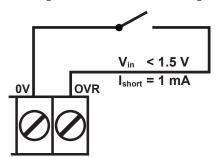
To provide output level override functionality, wire a switch between the '0 V' and 'OVR' terminals.
