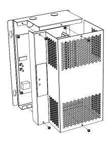
3. Remove the knockouts as required.
