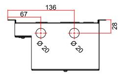
Knockouts: base (for power and output cables)
